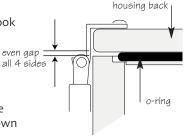
Double check - Once the housing is closed, check the o-ring seal. Check the gap between the housing back and the housing. It should be even all the way around the housing.
